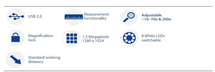
It is equipped with a high quality 1.3 Megapixels sensor with a crystal clear image quality and natural color reproduction, enabling you to view and capture objects with the greatest level of detail. This model comes with the DinoCapture 2.0 software for Windows and DinoXcope software for MacOS, allowing you to do calibrated measurements on pictures
